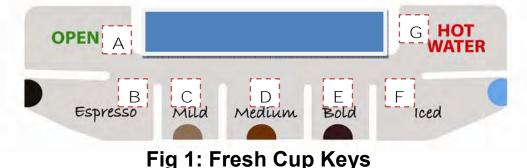
The Fresh Cup pod brewer has a menu that consist of scrolling menu entries that can be scanned through backward and forward using button A and button B (see Fig 1). To enter a programming record, press and hold the Hot Water Key (G) when powering up machine (see Fig 1) then use button A and button B (see Fig 1) to change the entry. Pressing the Hot Water (G) key (see Fig 1) will exit the entry, saving the entire Parameter structure to memory upon exiting
